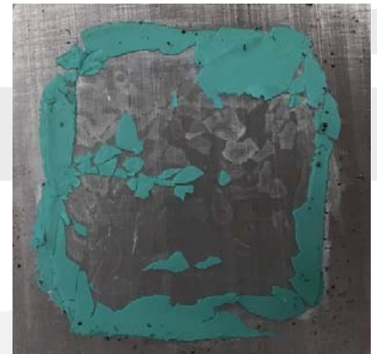
Below: Aluminum heat sink and thermal test module mating surfaces separated after thermal cycling.
