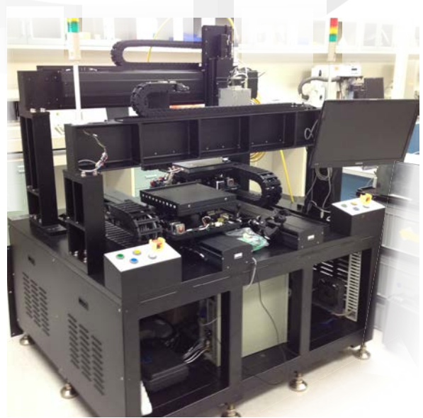
Laser selective reflow tool being installed in the APL.
