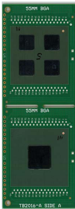
Lidless multi-chip and single chip FC-PBGAs assembled to a board.
