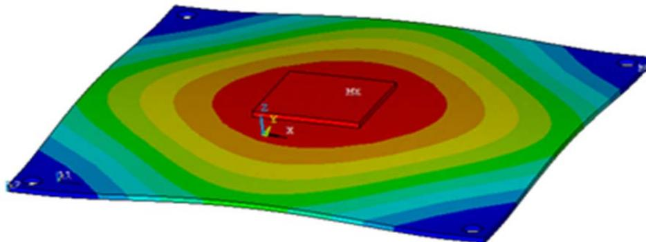
*First mode shape during natural frequency vibration of the VTV test board. Area of maximum deflection at the component site imposes cyclic solder joint strains and subsequent failure.*
