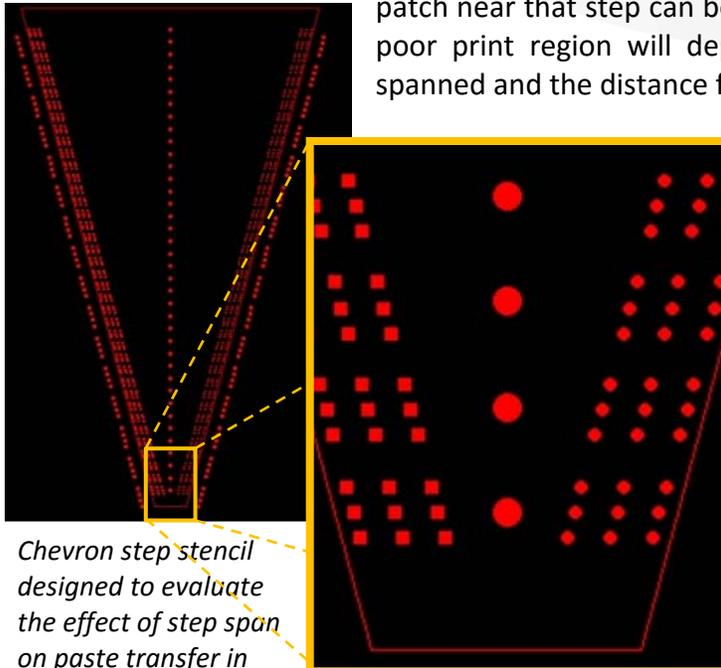
*Chevron step stencil designed to evaluate the effect of step span on paste transfer in close proximity to the step edge. Print direction is vertical.*
