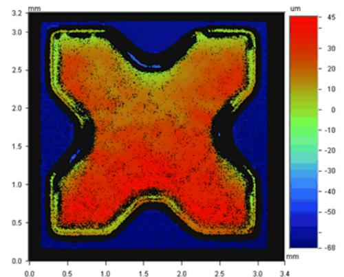
*Gradations in silver paste print deposit height as measured with the WYCO profilometer.*
