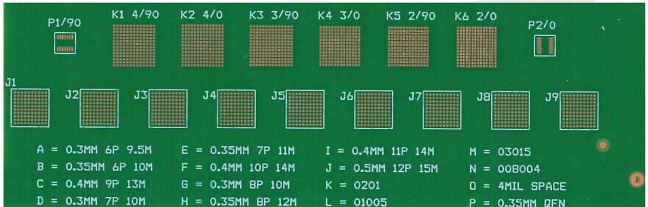
Upper and lower board edge segments of the Print Test Board 2016 enlarged to show fine pitch features.
