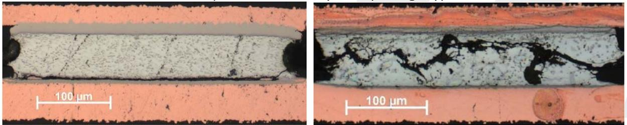
*LEFT: An experimental alloy solder joint with an interfacial separation along the ENIG board finish that produced an anomalously early ATC failure. RIGHT: A much later failure on the same ENIG board clearly arises from solder joint fatigue.*
