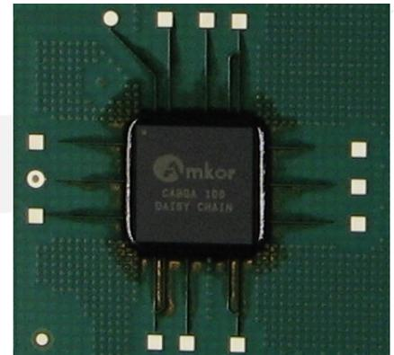
Thermal cycling of the prior TB2014U test boards with various underfilled components continues. The earliest group (underfills E and F plus non-underfilled controls) was removed from the chamber after more than 5500 cycles. The second group (underfills G and H) is still cycling and has now exceeded 3400 cycles. Failed parts have been cross-sectioned to identify failure modes.
