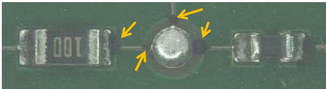
*A solder bead test point between 0603 and 0402 SMD resistors on a thin plasma coated board; a black creep corrosion product is visible growing on all exposed copper traces and surfaces.*
