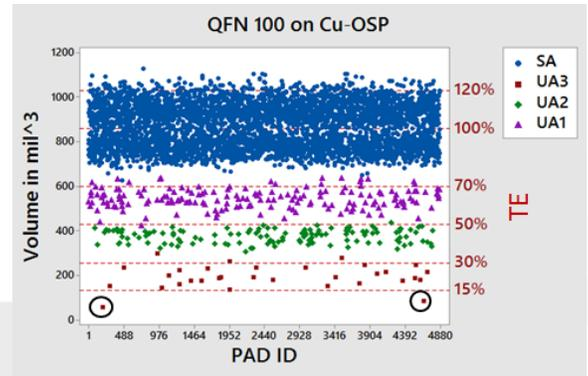
*Print volumes obtained with various Undersized Apertures (UA) relative to those with the Standard Aperture (SA) for QFN100. Circled points produced assembly defects.*
