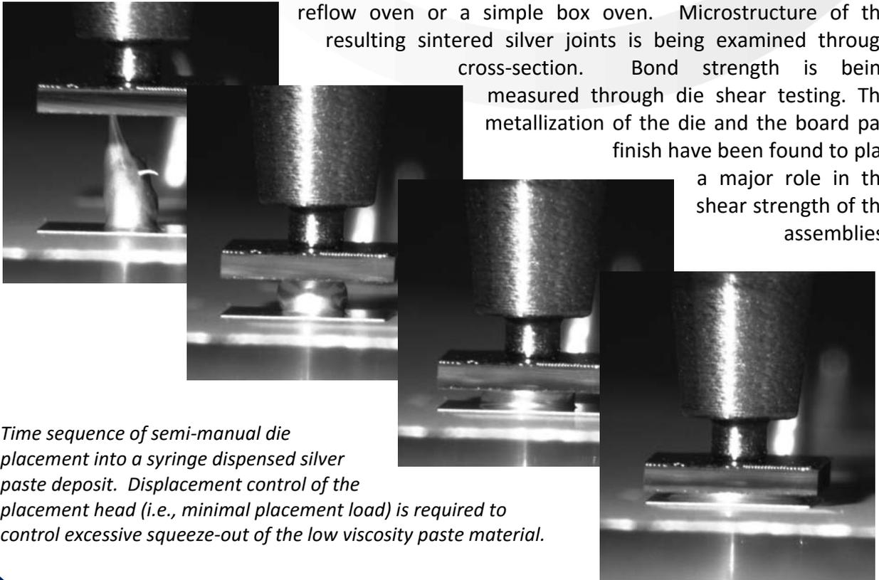
*Time sequence of semi-manual die placement into a syringe dispensed silver paste deposit. Displacement control of the placement head (i.e., minimal placement load) is required to control excessive squeeze-out of the low viscosity paste material.*
