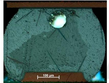
RIGHT: Cross-polarized optical image of the same joint revealing a multigrain Sn grain morphology.
