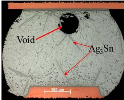
LEFT: Bright field optical micrograph of an **Innot** alloy BGA solder joint on Cu-OSP surface finish (board side) and electrolytic nickel-gold (component side).
