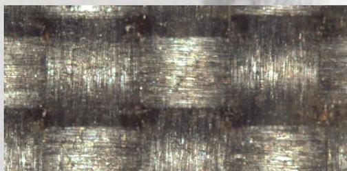
Hot Bump Pull strength measurements of PCBs with the same type of resins and identical pad design but from a new source are being taken, to investigate the difference between nominally similar substrates. Differences in strength were seen, which could at least partially be connected to differences in the glass weave. The analysis of the effect on strength of the pad location relative to the underlying glass bundles is continuing.
